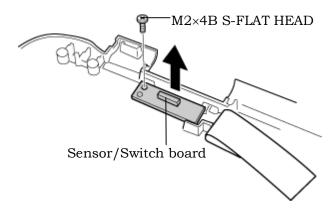
Figure 4-42 Removing the sensor/switch board
